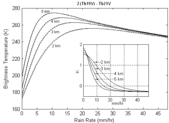
Fig. 1. Relation between brightness temperature (twice vertical polarization at 19.35 GHz minus 21.3 GHz) and rain rate at different freezing levels. The solid and dotted lines represent the relations for the preboost and postboost periods, respectively. The inset shows the difference in the  $T_b$ – $R$  relation in brightness temperatures between postboost and preboost orbital configurations.
