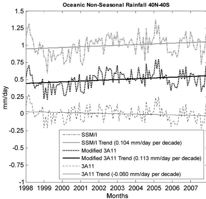
Fig. 5. Comparisons of linear-trend analyses of 3A11, modified 3A11, and SSM/I oceanic nonseasonal rainfall. The plots are shifted by 1 and 0.5 mm/day for SSM/I and modified 3A11, respectively.
