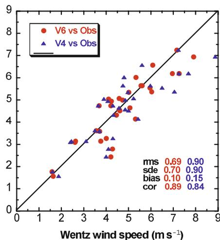
**Fig. 1.** The respective Wentz Version 6 (red solid circle) and Version 4 (blue solid triangle) (combined F13 and F14) daily surface wind speed vs the Kwajalein Experiment (KWAJEX) observed wind speed, adjusted for the surface, at  $9^\circ\text{N}$ ,  $167^\circ\text{E}$ , 28 July–11 September 1999.
