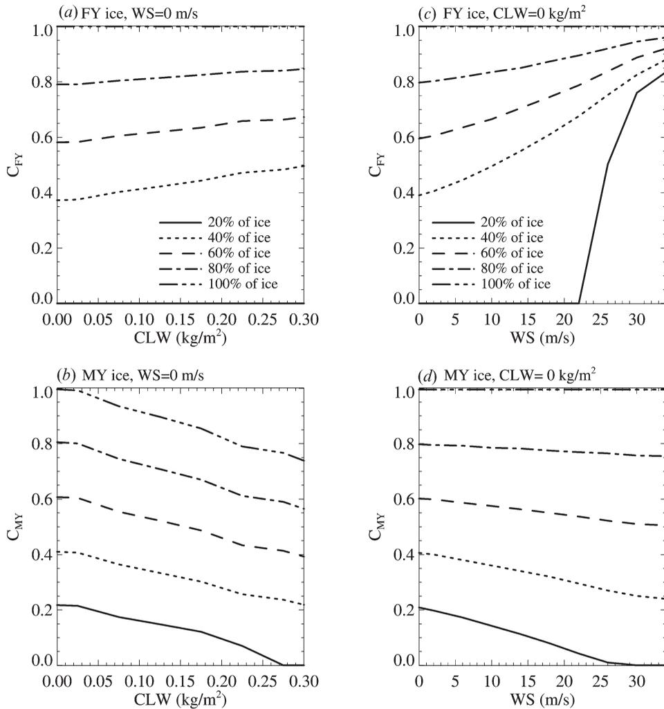
Figure 5. FY and MY ice concentrations ( $C_{FY}$ ,  $C_{MY}$ ) for each surface type as a function of (a,b) columnar cloud liquid water content (CLW) when surface wind speed (WS) is  $0 \text{ m s}^{-1}$  and as a function of (c,d) WS when CLW is  $0 \text{ kg m}^{-2}$ . The columnar water vapour (WV) content is fixed at  $2 \text{ mm}$  for both the cases.
