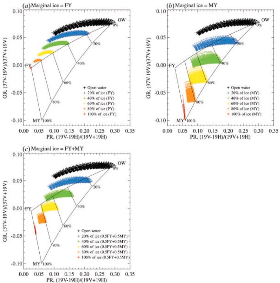
Figure 4. Scatter plots of the spectral gradient ratio (GR) versus the polarization ratio (PR) for the three different surface types: (a) open water (OW) and FY ice, (b) for OW and MY ice and (c) FY and MY ice. The fractions of ices are indicated by different colours. The triangle for ice concentration retrieval is superimposed. The lines of total ice concentrations are shown in 20% intervals.
